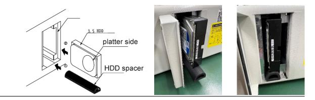
You can fold it in a V shape by using a rubber spacer.
