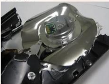
Destruction: Complete bending, and distortion of entire platter area leading to total data loss. This means that EVERYTHING and EVERY COMPONENT on a hard drive is targeted and demolished.
